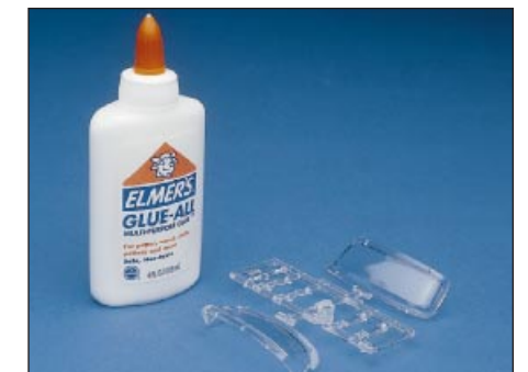
Attaching clear parts to a model can be tricky. Using too much regular model cement can soften and distort the parts, and superglue can "frost" their surfaces and ruin them. Water-based glues like Elmer's Glue-All and Microscale's Micro Kristal Klear are great for attaching clear parts; they're stronger than you'd think, they won't harm the plastic, and any excess glue is easy to clean off with a cotton swab and a little water.
