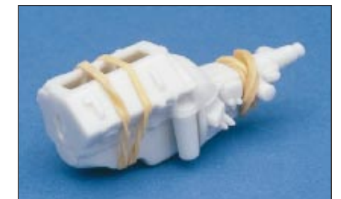
Rubber bands are one of the handiest (and least expensive) modeling tools you'll find. During assembly, they'll hold parts together securely while the cement dries.
